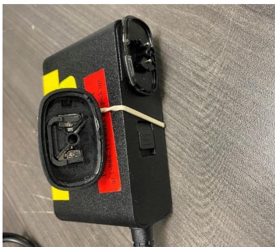
Figure 2: Damaged Input Plug
