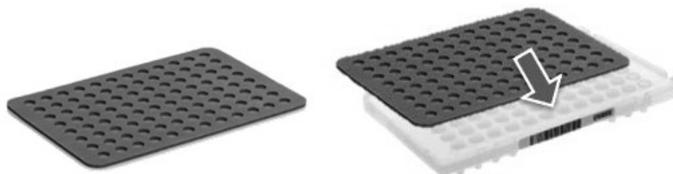
Figure 1: MicroAmp Optical Film Compression Pad (left) and placement of the Compression Pad on a 96-well MicroAmp Reaction Plate (right). The gray side should always be placed down and the brown side up.
