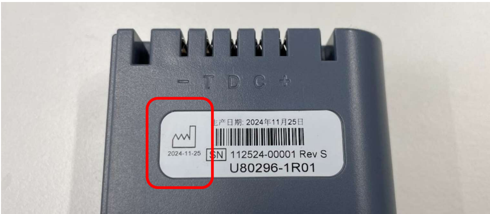
Figure 2. Example label of an affected battery. Contains Part Number “U80296-1R01”, Revision “Rev S”, manufacturing date “2024-11-25” located under the date of manufacture symbol.
