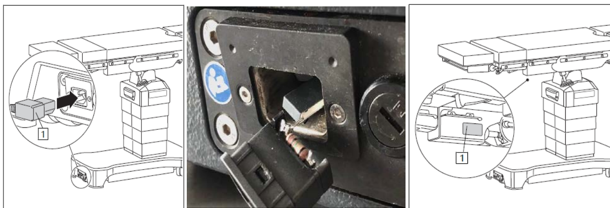
Figure 1: Position mains connection on OR-Table / pulled out mains connection with exposed electronic components / position of product label on mobile OR-Table MEERA including SN
