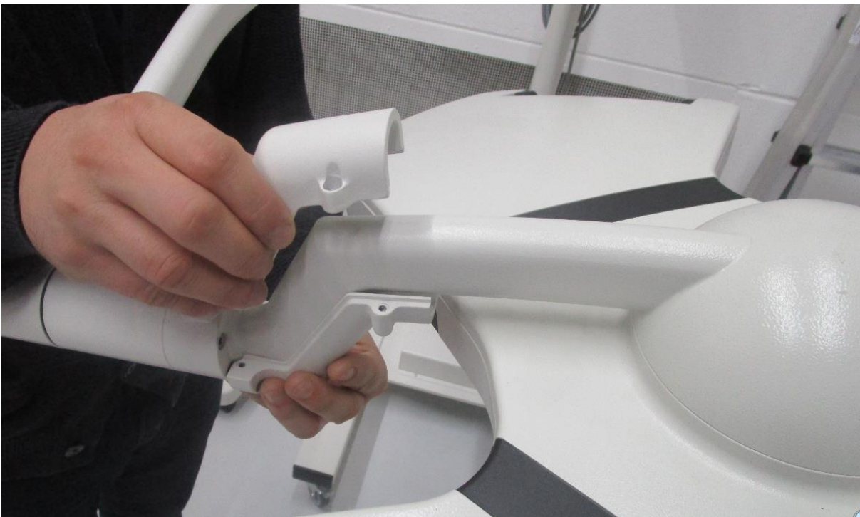
Figure 4: Installation of the safety device set
