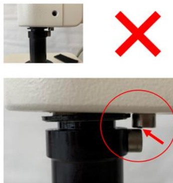
Figure 5: Detailed view of stopper screw when M220 F12 is faulty: Stopper screws are not effective and allow free rotation > 360°. → Immediately stop using the device! The M220 F12 can no longer be used.
