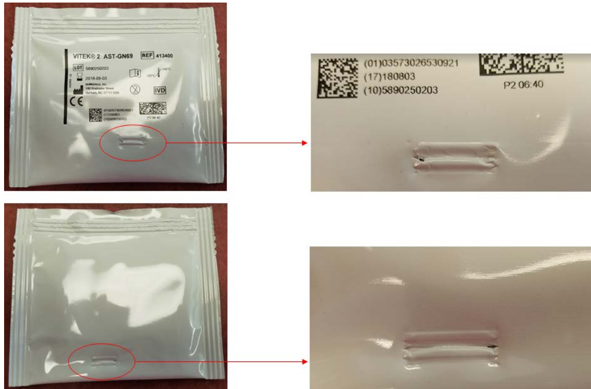
Figure A - Example of Pouch Defect
